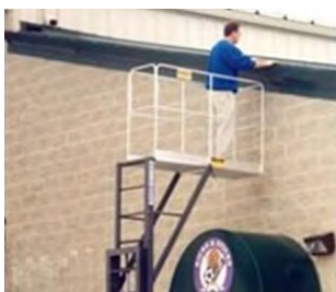
Cantilevered platform extends 34" beyond base frame
