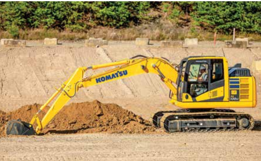
With more track on the ground than its predecessor, the PC130LC-11 has greater lift capacity.
