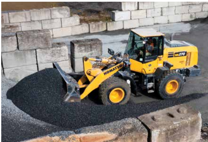
At one of Blue Dot Readi-Mix’s eight state-of-the-art facilities, an operator scoops material with a Komatsu WA270-8 wheel loader.
