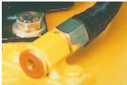
The oil drainage pipe makes oil changes simple and easy
