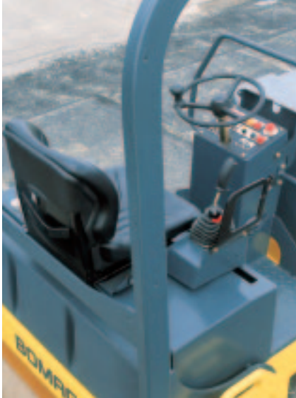
Ergonomic control layout for simple operation
