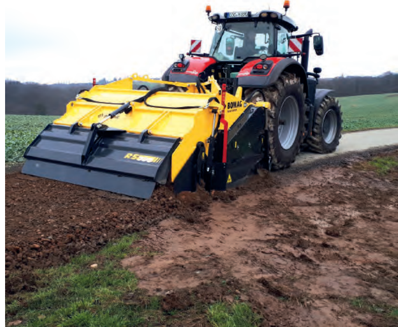
The RS 300 has height-adjustable side plates, including skids, with a free, hydraulically, adjustable milling depth up to 50 cm
