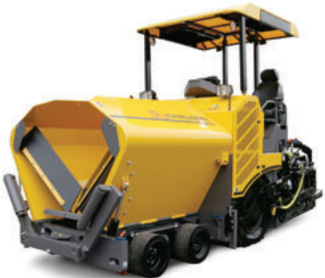
Carlson’s CP65 City Paver delivers laydown rates of up to 250 tonnes per hour.
