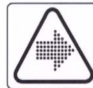
Air/gas flow or Air discharge.
