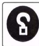
Tie down point
