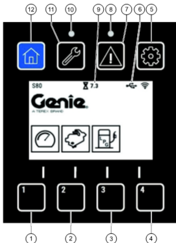
ALC-600 Control System Display
