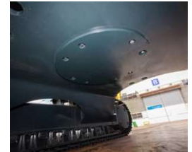
2 Pieces of Under-cover can help easy maintenance.
