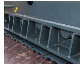
Heavy Duty Track with Full Track Guard installed.
