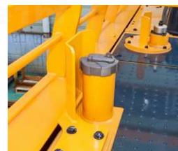
Fuel and Hydraulic Oil inlet can be protected from the harsh site condition.
