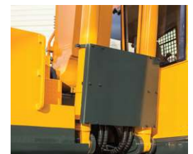
Boom Cylinder Guard can protect them from the harsh site condition.
