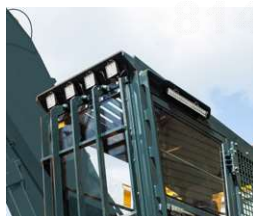
Cabin Lamp as LED style for customer satisfaction with side lamp additional.
