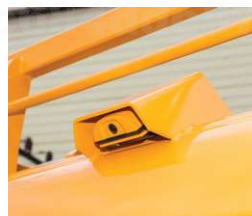
Rear Camera is fully protected by welding type protection plate.
