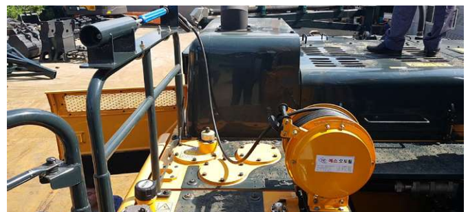
Self Cleaning Hose installed
