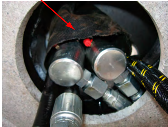
Viewed looking up from crane box. The pressure, return, and rotation hoses are wrapped in the 60350105 hose sleeve.
