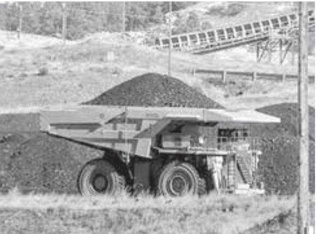
Custom-built truck bodies have a large body to accommodate coal's natural properties and are designed to keep one-third of the weight on the front of the truck and two-thirds of the weight on the back of the truck.
