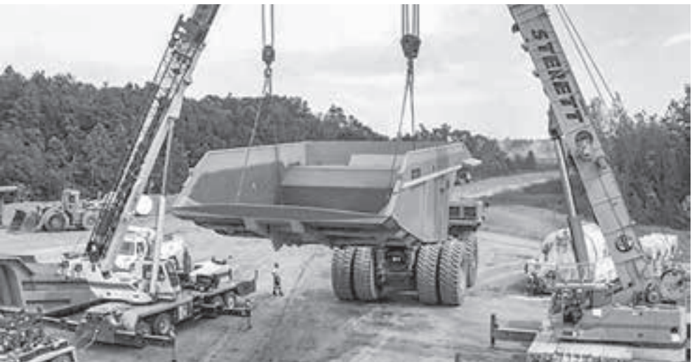
Customized haul truck bodies, such as these designed by Philippi-Hagenbuch, can increase productivity by taking into account specific load characteristics.
