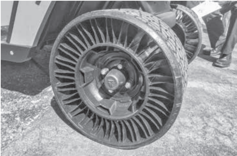
At Movin' On 2017 in Montreal, Michelin unveiled VISION, its new concept tire that is airless, customizable and both a wheel and tire.
