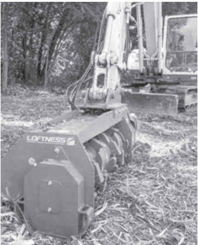
The new Battle Ax mulching attachment by Loftness is available with 41-, 51- and 61-inch cutting widths.
