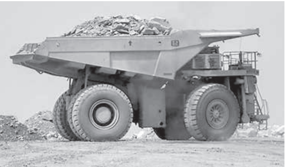
Overburden materials vary among mines, which is why engineers scrutinize material information, including 3D scans, photographs or video, from each mine to determine the best truck body design for that application.
