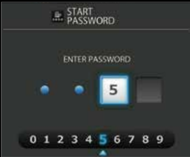
Engine start password A password is required when starting the engine for greater security.
