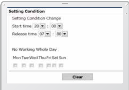
Engine start alarm outside prescribed work time
