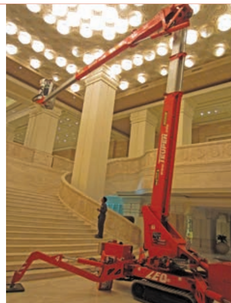
A Teupen Leo 23 GT belonging to MTandt negotiates a staircase.
