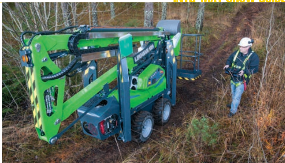
The Leguan 135 includes a range of new features that provide easier, safer and more efficient operation. The dual-power machine provides 13.2 m vertical and 6.8 m horizontal reach.
