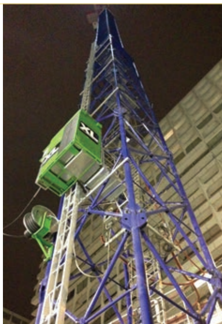
XL's X-Up 200 is a rack and pinion construction elevator specifically designed for tower cranes.
