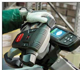
Multifunctional steering wheel with optional color display.
