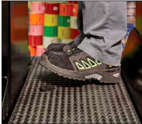
Foot switch for lowering the driver's platform
