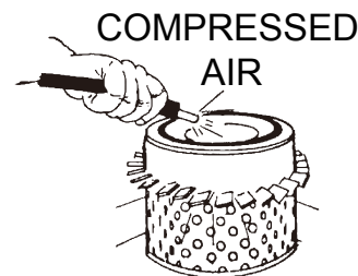
Figure 23. Cleaning Air Cleaner Element
