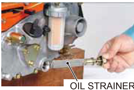
Figure 21. Engine Oil Draining
