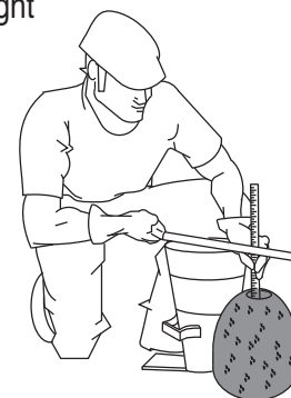
Figure 54-F. Slump Test (Measurement)
