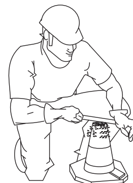
Figure 54-D. Slump Test (Removing Excess Concrete)
