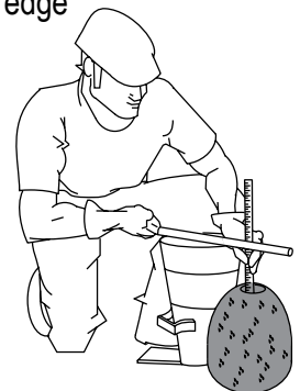
Figure 54-F. Slump Test (Measurement)
