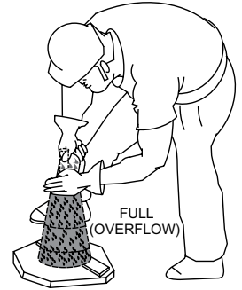
Figure 54-C. Slump Test (Full-Overflow)
