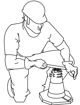
Figure 54-D. Slump Test (Removing Excess Concrete)
