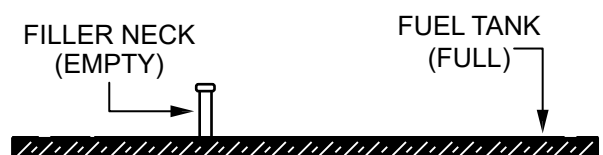
Figure 31. Full Fuel Tank
