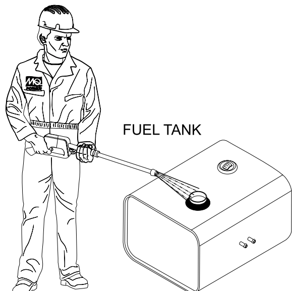
Figure 45. Fuel Tank Cleaning
