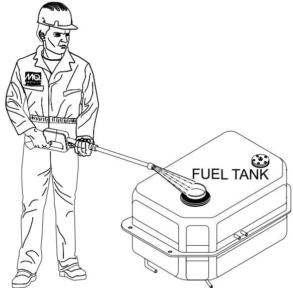
Figure 60. Fuel Tank Cleaning
