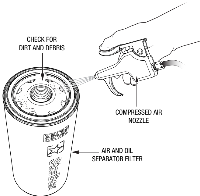
Figure 27. Air and Oil Separator Filter Inspection and Cleaning
