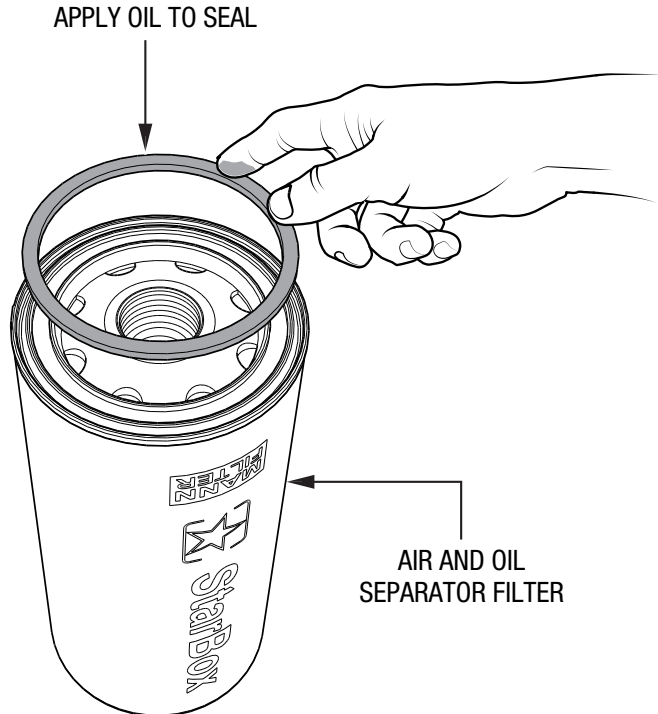
Figure 28. Air and Oil Separator Filter Seal Lubrication
