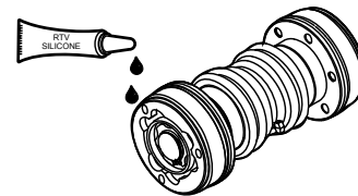
Figure 29. Applying RTF Silicone
