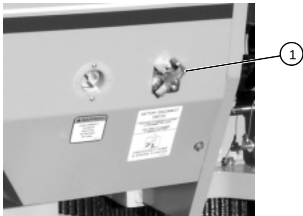
Figure 2-2. Battery Disconnect Switch
