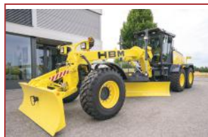
HBM BG 190 Motor Grader (New) 19.00 tonne, EROPS/FOPS cab with a/c, LED lights, 3.6m blade, rear rippers, Michelin tyres. Available in 6 x 4 or 6 x 6 configuration. Impressive German quality graders – call for pricing.
