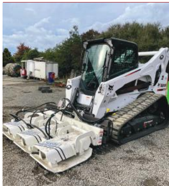
STEHR SBV80HC3 TRIPLE PLATE COMPACTOR 2.120 mm working width, 70Hz Frequency, Centrifugal Force 3 x 80kN available with either an independent PTO Power Pack or able to be fitted to suitable Skid Steer Loaders. Ideal for working in sensitive areas, close to buildings etc. A versatile & productive unit. WINTER TIME SPECIAL PRICING FOR STOCK UNIT. SAVE $'S ON INDENT PRICING.
