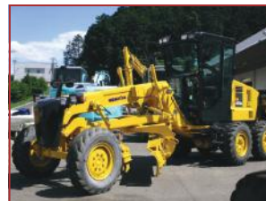
KOMATSU GD 405A-3 MOTOR GRADER YOM 2008, 3.875 hours, cab with a/c. 3.100m mouldboard, front scarifiers and front push block. Tidy compact grader, very tidy.
