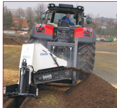
STEHR SGF 1300-350 TRENCHER for attachment to Ag Tractors, PTO Driven. Max cutting depth 1.300 mm, cutting width 350 mm. An impressive machine. Demonstration unit available with WINTER TIME SPECIAL PRICING.
