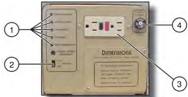
Figure 3-9. 1500W AC Inverter
