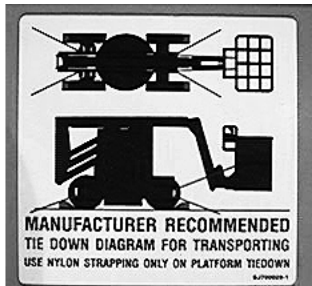
Figure 2-10. Recommended Tie Down Locations
