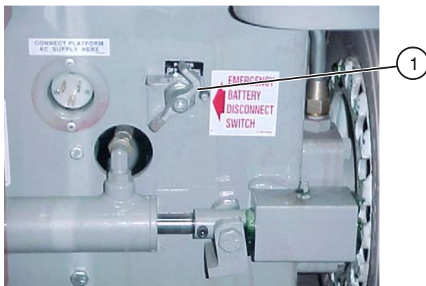
Figure 2-2. Emergency Battery Disconnect Switch
