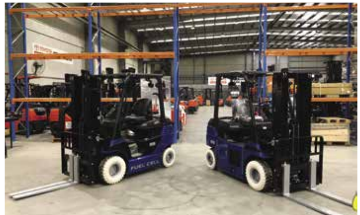
Toyota hydrogen FC forklifts have a nominal rating of 2,500kg lift capacity
