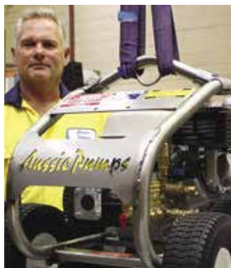
Aussie's new 3,000psi compact 'hire spec' high pressure cleaner
