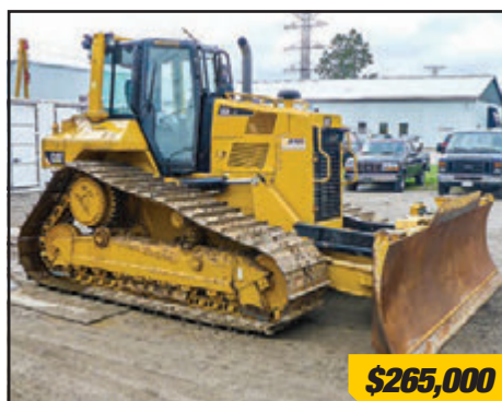
CAT D6N LGP (2016) - 3,835 Hours 6 Way PAT Blade, Ripper Ready, Rear Auxiliary Hydraulics, Accu-grade Ready, SALT Undercarriage, 33" Pads, Warranty.
